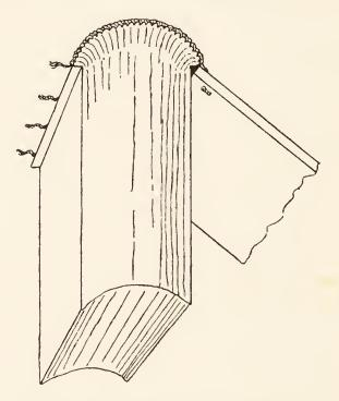
FIG. 2.—Rounded Back of sewn book before the side boards are attached
